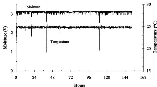
**Figure 2.** Representative environmental control of moisture-maintained experiments under continuous irradiation. Data are from the iron-fortified experiment.
